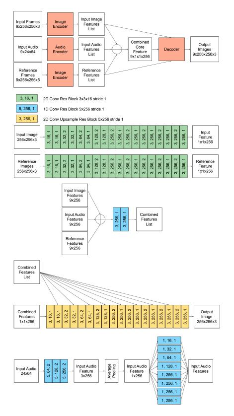
Figure 8 | Network architecture: the first row shows the overall architecture, and the pieces below show constituent component details.
