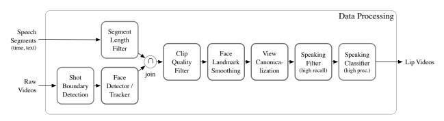
Figure 3 | Data collection and filtering pipeline.
